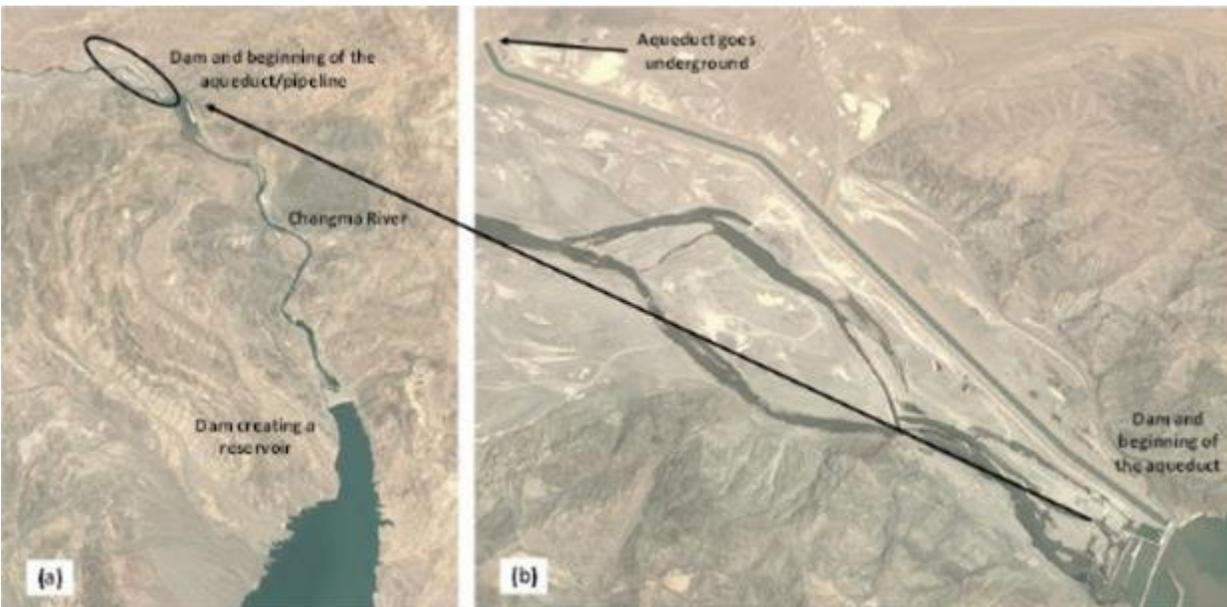
**Figure 6. Likely location of the beginning of the aqueduct and pipeline carrying water from the Changma River, roughly southwest of Yumenzhen, to the 404 Plant. The locations are 50-some kilometers from the plant, as described in the blog of a former worker. (a) An overview, and (b) a closeup of the beginning of the aqueduct and pipeline.**
