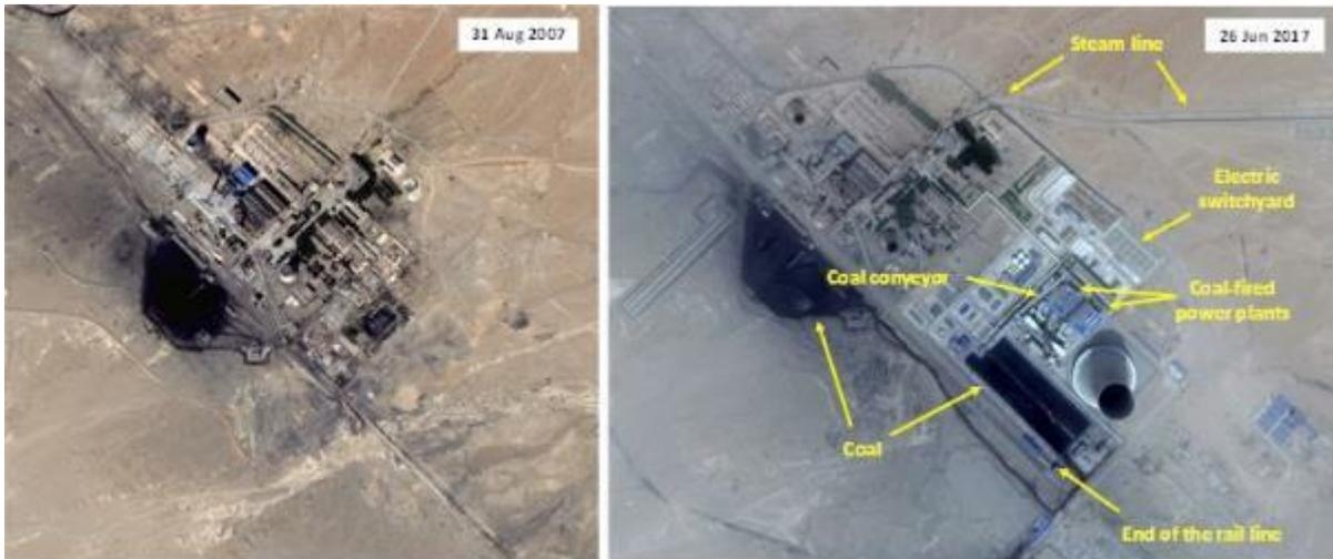
**Figure 11. Expansion of the coal-fired electrical generation capacity at the 404 Plant site, in an area near the reactor and reprocessing area. One can see that the new cooling tower is much larger than the existing cooling towers in the area. The smaller cooling towers are comparable in size to the six cooling towers used by the reactor.**
